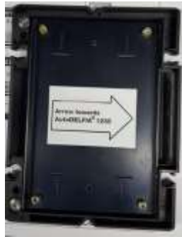
Fig. Search Plate – it is used in a measuring unit to calibrate the positions of microplates so that they can be lined up for detection
