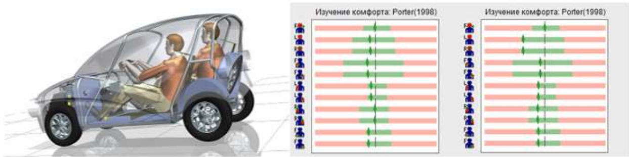
Evaluation of 3D-dummies: driver (left) and passenger (right). A zone of discomfort is shown in red on the histogram.
